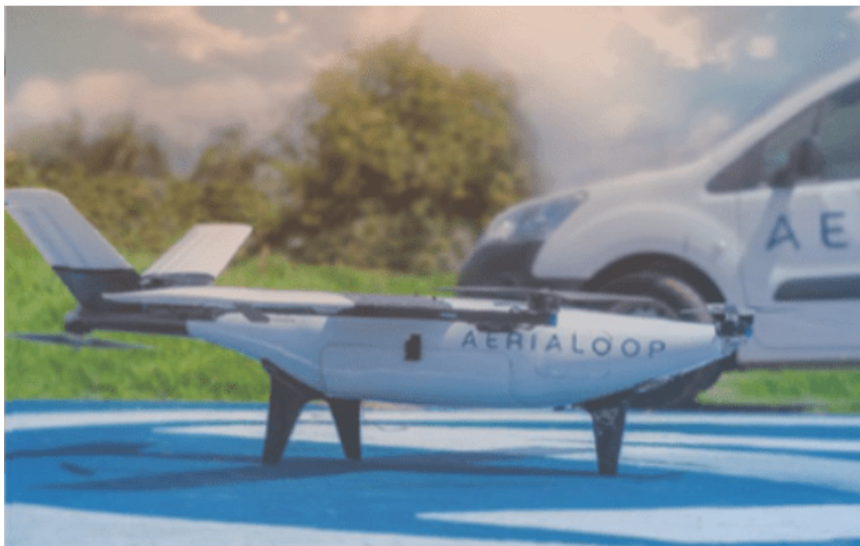
Aerialoop’s ALT6-4 VTOL Delivery Drone is 6 feet long, battery powered and capable of carrying almost 9 pounds. (Courtesy image | Aerialoop, City of Arlington)
