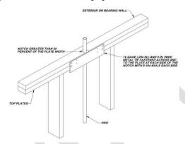
(Amendment to 2015 IRC carried forward to 2018 IRC also provides additional assurance of maintaining the integrity of the framing by spreading the nailing pattern.)
