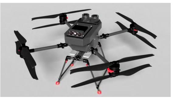
Custom built carbon fiber airframe by XM2
