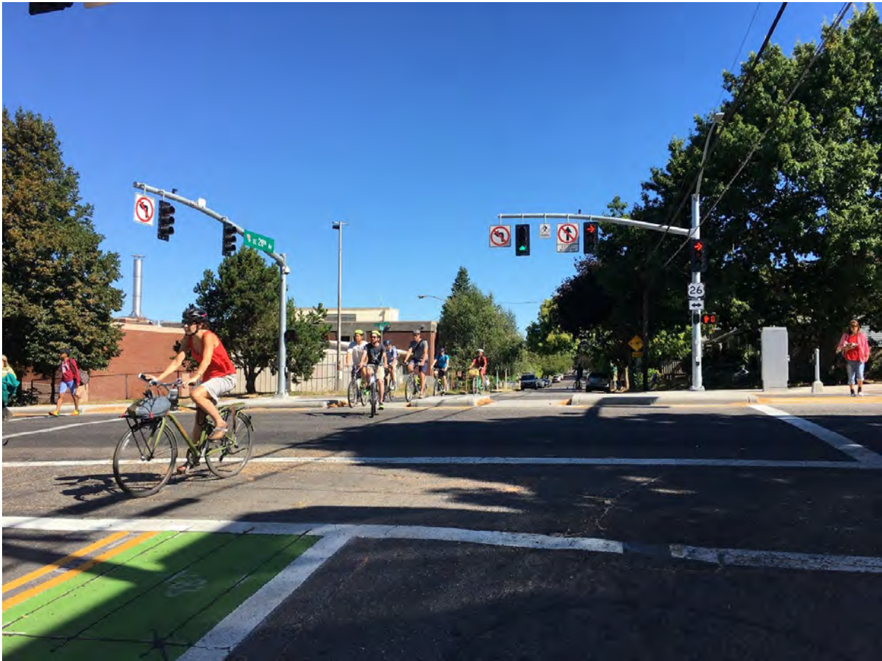
A median island refuge at an intersection serving as a diverter allows bicyclists to comfortably travel across three or more lanes while also reducing through traffic.
