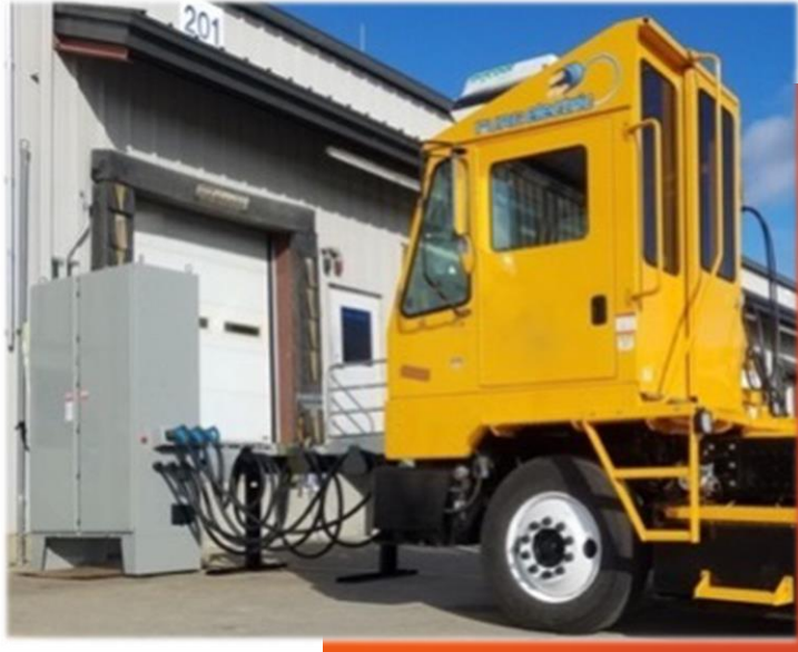
Orange EV Fast Offboard Charging Cabinet: Up to 70 kW
